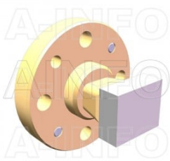
LB-5-15-ASPO Standard Gain Horn Antenna 140-220GHz 15dB Gain Rectangular Waveguide Interface
